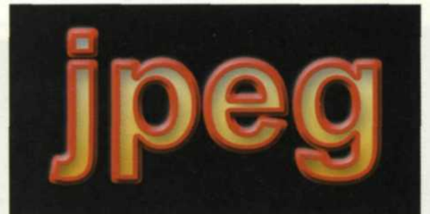
Original test file created in Adobe Photoshop 6.0. Text was converted to bitmap and saved as an uncompressed tiff file.
